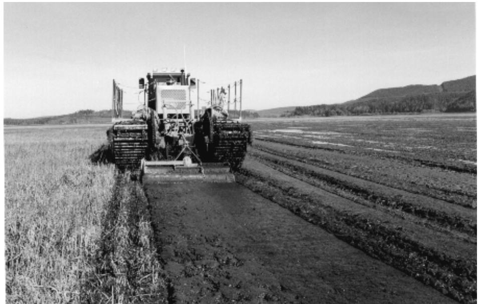
The Refuge's Wilco amphibious tractor/rototiller plows a spartina meadow at the Porter Point Unit to prevent root spread.
