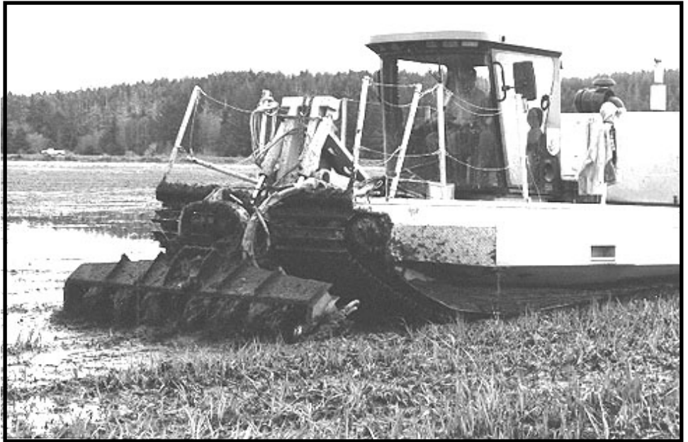
The Refuge's amphibious tractor with a rototiller attachment rigged in place of the conventional mower cuts spartina roots to prevent spread of the infestation.
